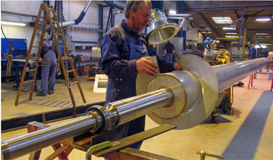
Screw rotor with centerpipe st.52.
